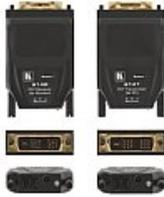
The 614T and 614R are a small and lightweight, detachable optical transmitter and receiver pair. They transmit uncompressed DVI resolutions of up to 1920x1200 at 60Hz using one multimode fiber optic cable with SC connectors. The 614T converts the DVI signal to an optical signal that it transmits to the 614R. The 614R decodes the optical signals back to a DVI signal.
